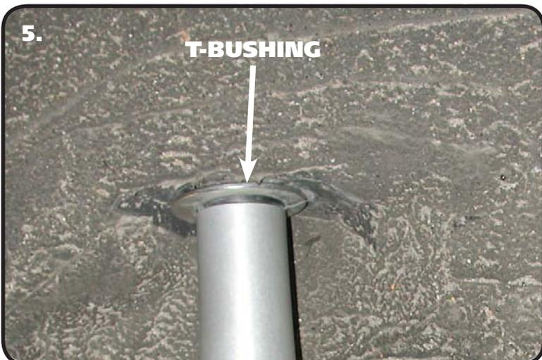
5. **Image 5** illustrates how the T-Bushing is installed.
