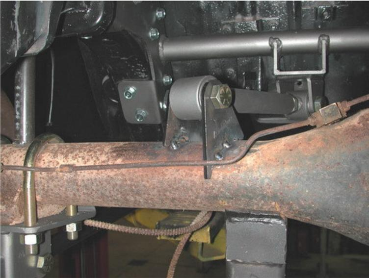
15. Check the length of the upper bar; it should be 10" C-C. Bolt the axle tabs to the upper bar with the larger tab to the inside. Then place the other end into the bridge. Both ends use a 5/8" x 2 3/4" and should not be fully tightened yet.
