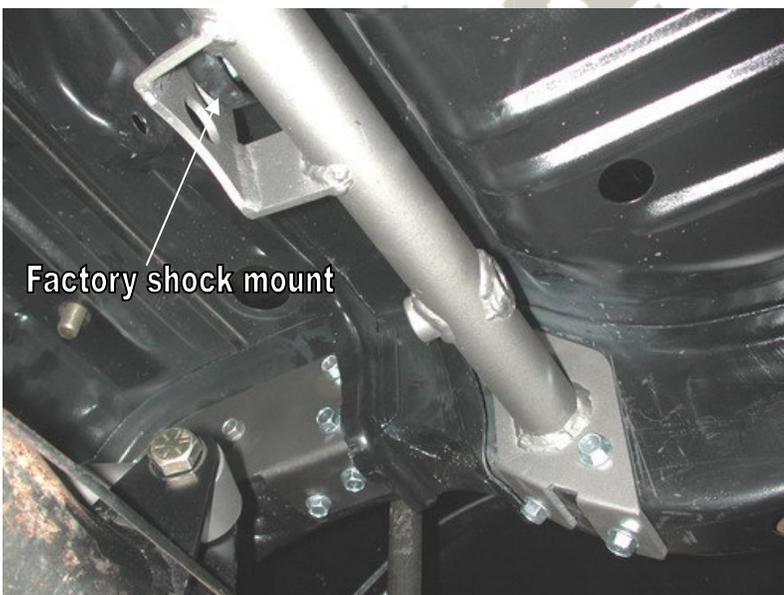
5. The upper Shockwave bridge will slide between the frame rails directly behind the factory shock cross member. The bridge will be positioned by bolting the tabs to the factory shock hole. Fasten the bridge to the factory shock mount using 1/2" x 1 1/2" bolt, flat washer and Nyloc nuts. Using the bridge as a template drill the holes in the frame with a 5/16" bit. 3/8" x 1" thread forming bolts and flat washers will hold the bridge in place.
